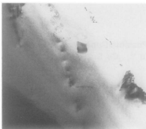
FIG. 1. Electron micrograph of a large piece of crystal ($1) of YSr_2(CuFe)_3O_{6+z} showing either a dislocation or a sub-grain boundary ( \times 42,500 ).
